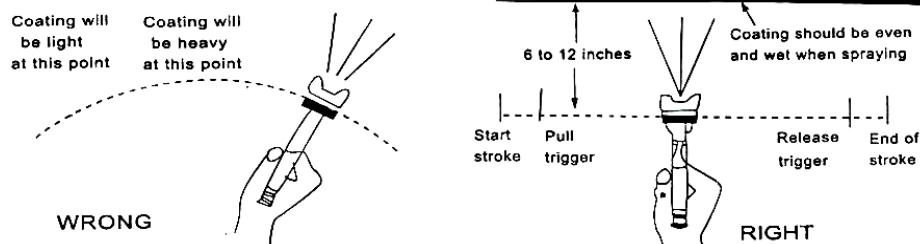
2. Where possible, avoid stopping and starting when spraying an object. This can lead to too much, or not enough paint being applied. Never start or stop the spray gun while it is aimed at the surface to be sprayed.
